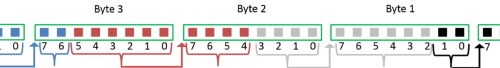
Figure 1. Packing two 10-bit pixels into three bytes.
